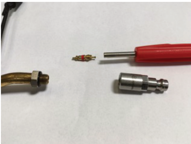
IMG 5: Tear out the standard valve core
