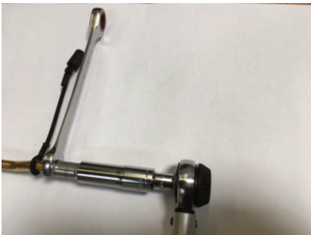
IMG 8: Fix the groove nut with a wrench 11mm and turn the Tire Valve Connector with a long box nut and a torque of 6Nm against the groove nut. Make sure the O-ring is in the right position.
