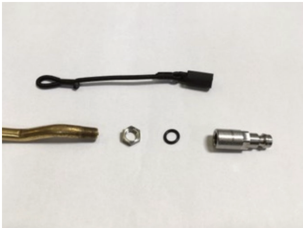
IMG 1: Components of the Tire Valve Connector
