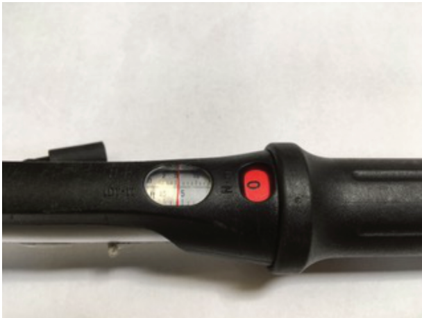
IMG 7: Adjust the torque wrench to 6Nm
