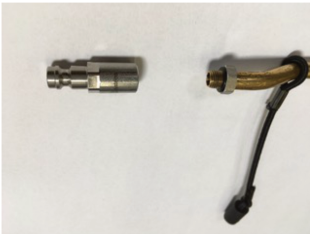
IMG 4: Push the O-ring against the groove nut
