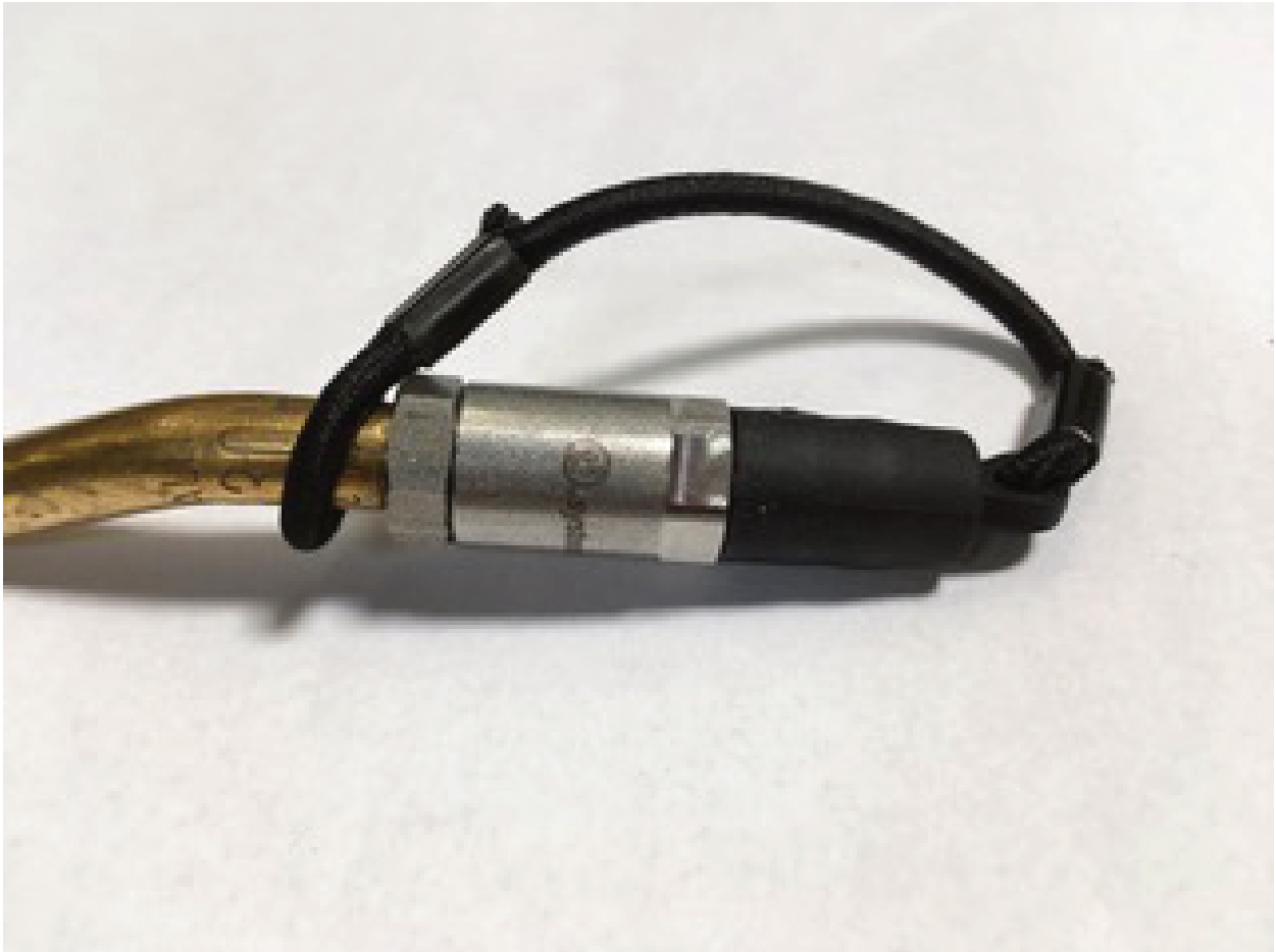
IMG 9: Tire Valve Connector. After installation and under pressure, test referring to any leakage with a liquid leak finder. If there should be any leakage, the torque can be increased up to 7Nm. After testing and cleaning, put the protection cover onto the Tire Valve Connector.
